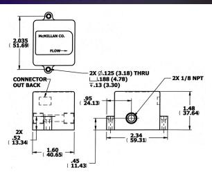
Dimensions shown are in inches(mm) and do not reflect included fittings. Dimensions shown are for the Model 104 and are similar for other models. Specific dimensional drawings for each model may be requested from the factory.
