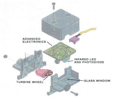
erated. Consequently, zero drift is not possible and zero adjustments are never required. Processing circuitry provides analog and/or pulse outputs that are linearly proportional to the flow rate.
