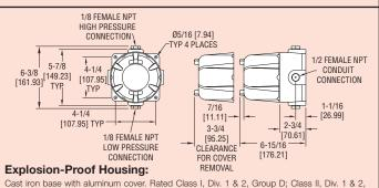
Groups E, F, G; Class III and NEMA 7 CD, 9 EFG. Wt. 7½ lbs. (3.4kg). Switch must be factory installed. Change base number to 1824 and add -EXPL suffix. Example: 1824-1-EXPL
