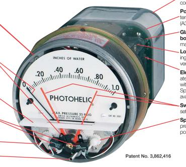
Plastic enclosure protects electronic components and electrical connections.
