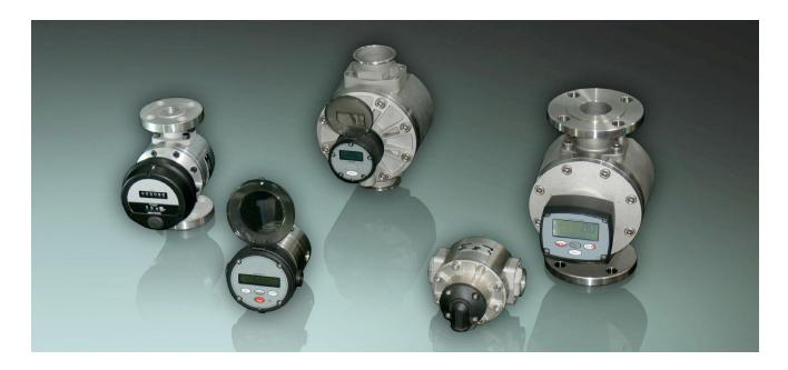
Fluidex series MOGF is a Positive Displacement Flow Meter with medium capacity. The meters have two rotating gears in oval-shape. A fixed amount of the liquid passes between the gear teeth and through the meter after each revolution. The flow rate is identified by the number of shaft rotations. MOGF are used in a wide range of applications where accurate measurement of liquid is required.
