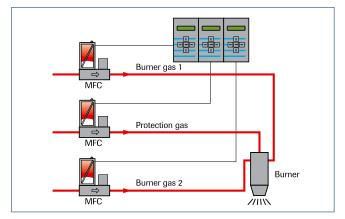
Burner control using Mass Flow Controllers brings many advantages compared to conventional systems, where flow is adjusted through needle valves. When burner orifices get clogged or when gas supply pressure varies, an MFC will automatically adapt to the changed conditions. For the control of relatively large flows with low differential pressure, which is typical for natural gas or  $CH_{4^{+}}$ . Bronkhorst High-Tech offers mass flow meters with separate pressure compensated bellow valves.
