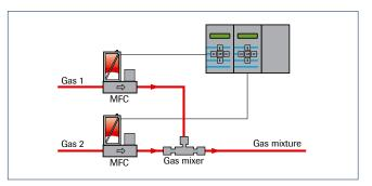
MFC's are often used to make precise and stable mixtures of two or more gases. A Bronkhorst PS/Readout system can be applied to maintain the ratio of mixed gases by operating in master-slave mode. In the example above, the flow range of gas 1 is much smaller than the other. For this purpose Bronkhorst High-Tech developed a gas mixer, to guarantee a homogeneous gas mixture.
